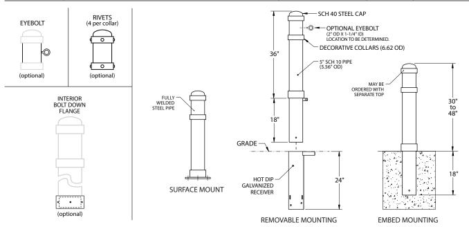
B-1 Bollards shown above in 5" pipe, also available in 8" dia. and in 30", 36", 42" and 48" heights, removable bollard receivers sold separately.
